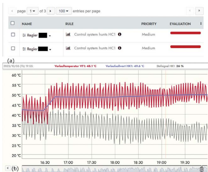
Figure 6.13: Example of predictive maintenance of a substation. Part (a) depicts a real predictive maintenance warning. Part (b) depicts values from the corresponding substation: valve position is shown in grey, secondary inlet temperature in red and setpoint secondary inlet temperature in purple. This substation shows strongly oscillating control, leading to fatigue of elements such as the actuator of the controller.
