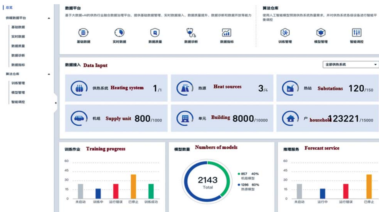
Figure 5.29: The dashboard of a typical smart DH control platform in China
