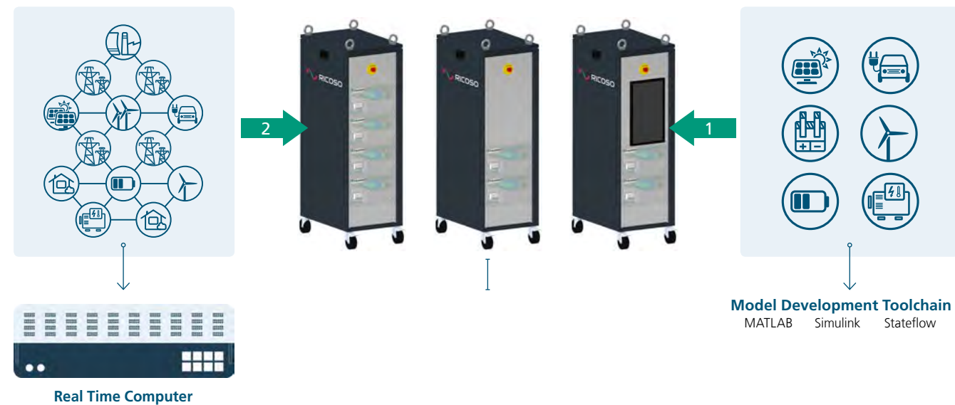
Figure: Using the RICOSO system as Rapid Inverter Prototyping Solution (1), Power Hardware- in-the-Loop (2)
